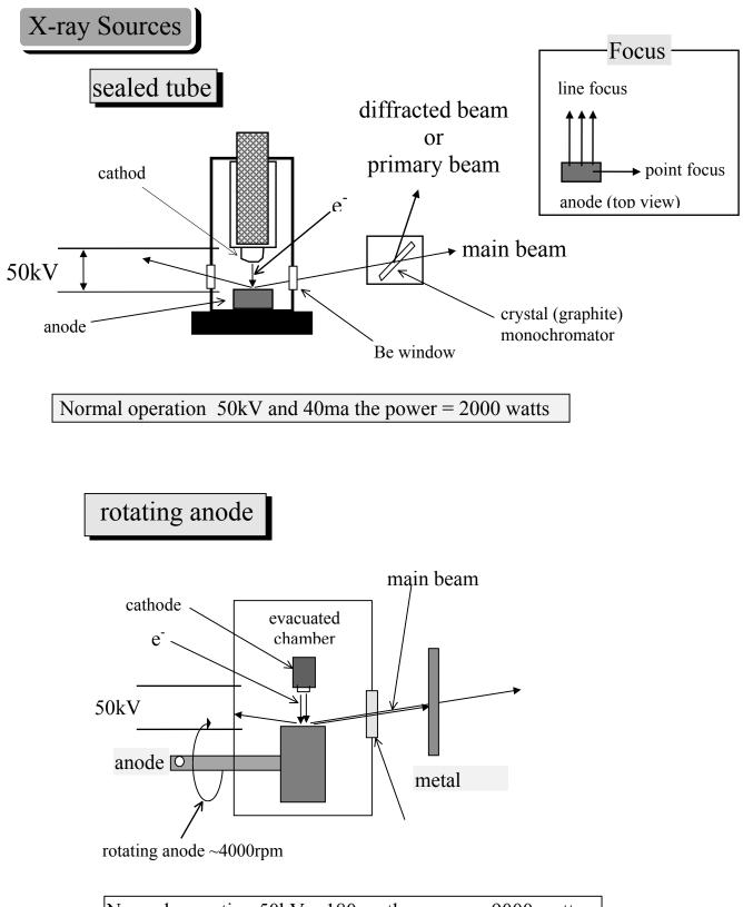
Normal operation  $50 \text{kV} \times 180 \text{ma}$  the power = 9000 watts
