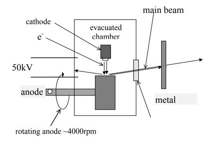
Normal operation  $50kV \times 180ma$  the power = 9000 watts
