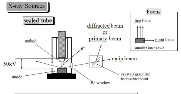
Normal <u>operation 50kV</u> and 40ma the power = 2000 watts
