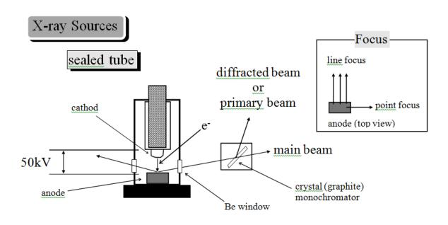
Normal operation 50kV and 40ma the power = 2000 watts
