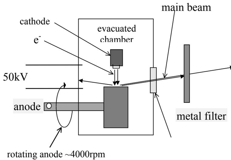
Normal operation 50kV x 180ma the power = 9000 watts
