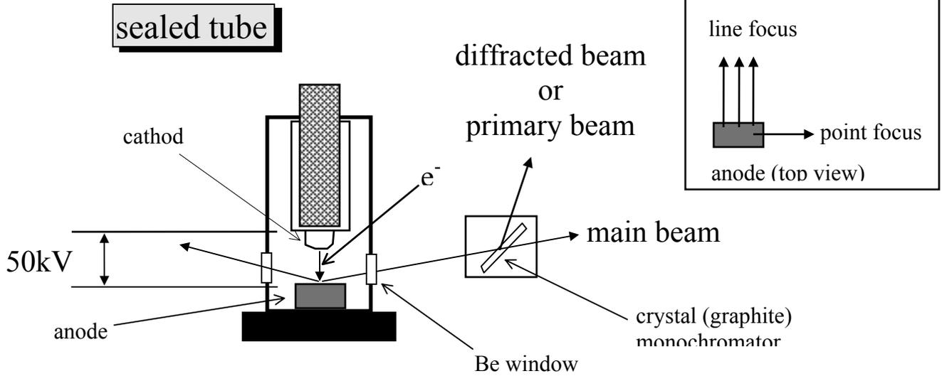
Normal operation 50kV and 30ma the power = 1500 watts
