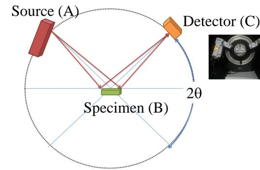
BRAGG BRENTANO :The detector is positioned at  $2\theta$  angle to collect the data. The number of X-rays counted by the detector is proportional to the intensity (I) of the scattered X-ray
