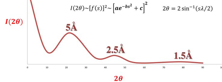
For a linear ordered system where the same element (atom) is spaced at equal distance(s) of  $a$   $N > 2$  times then
