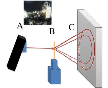
Transmission with Area detection. The area (2D) detector is positioned behind the sample. X-rays travel through the sample and are collected at the detector
